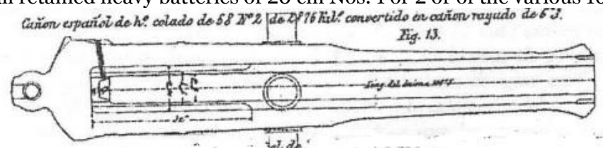
Fig. 27. Section 20cm No.1 Palliser conversion to 16cm No2 (Calvo, 2014)
