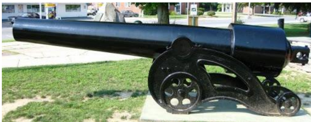
Fig. 23. Parrott 100 pdr 6.5-inch gun showing 'light' cast-iron barrel and short reinforce
