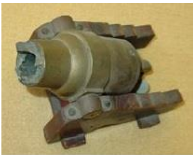
Fig. 56. Spanish gun failure due to compressed powder
