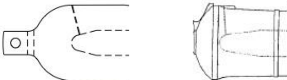
Fig. 32. Breech and chamber of Dahlgren 9in SB
