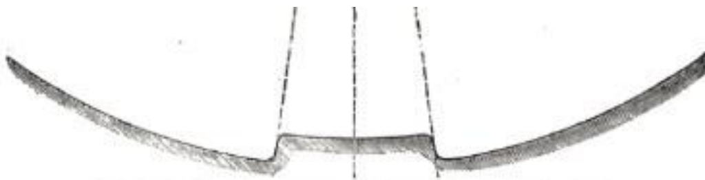
Fig. 22. Vavasseur MLR rifling from Mechanics
