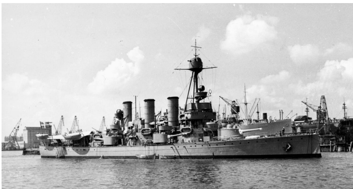
Fig. 6. «Oscar II» in Gothenburg 15 July 1946. A rangefinder is seen on her fighting top, life-floats are attached to the superstructure and the radio directionfinder antenna has been moved to forward of the searchlight platform (photo is courtesy Curt S. Ohlsson)
