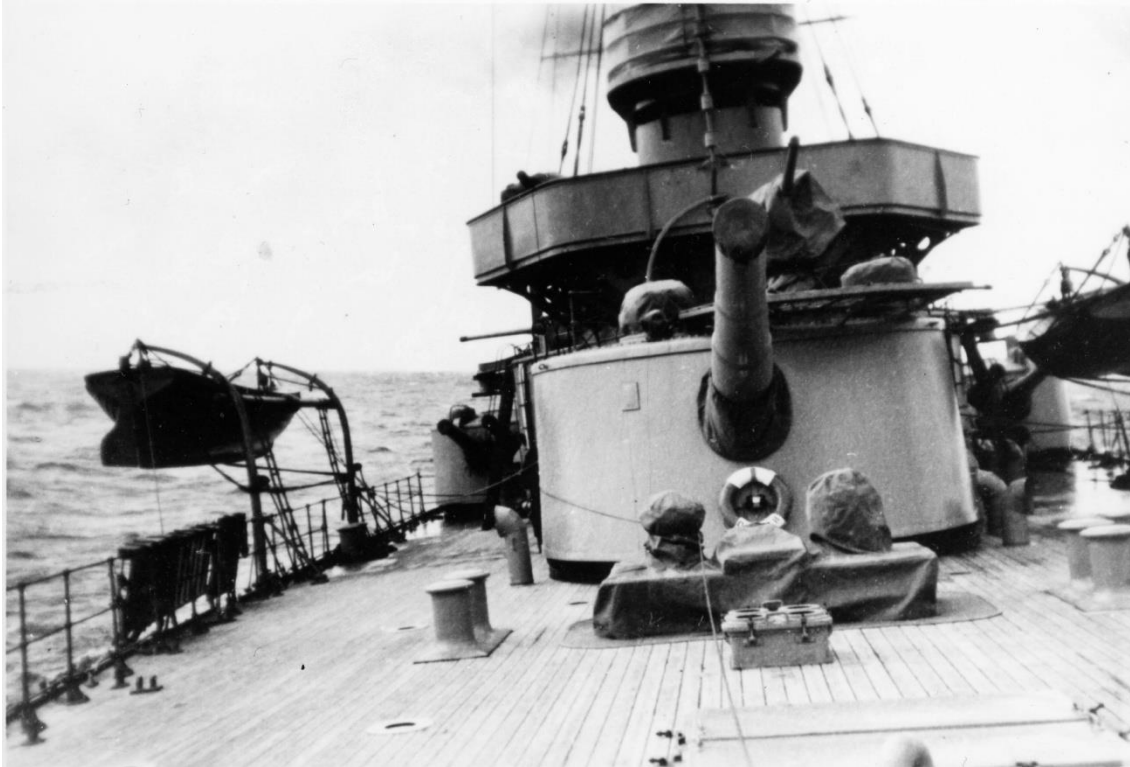
Fig. 3. The after 21 cm gunturret. The barrels of the after 57 mm guns are also visible
