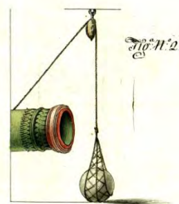
Figure 3. Scale comparison of a 3-kantar and a 1-kantar barrel (above) and the cutaway view of a 3-kantar barrel; together with the sling and pulley system to handle the enormous 336 pound marble ball (below) These drawings are part of a Venetian spy report from 1725
