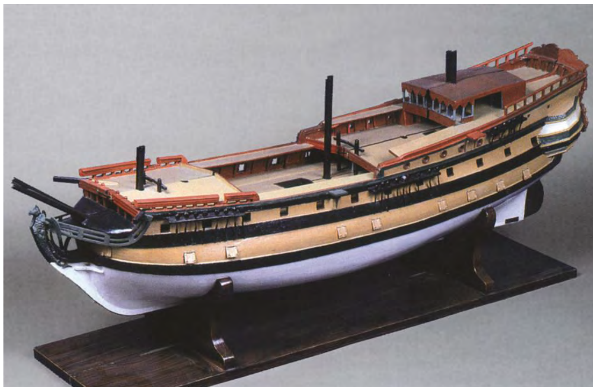
Figure 2. The photo of the Ejder Başlı/Leontii Muchenik 's exquisite dockyard model, currently in the collections of the Central Naval Museum in St. Petersburg. This model was for long thought to represent the « Semend-i Bahri », a similar 60-gunport ship captured at the battle of Chesma and renamed as « Rodos » by the Russians
